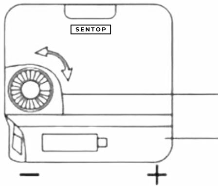
A rotating mechanism on the back of the clockwork, with which you can set the correct time on the wall clock.
